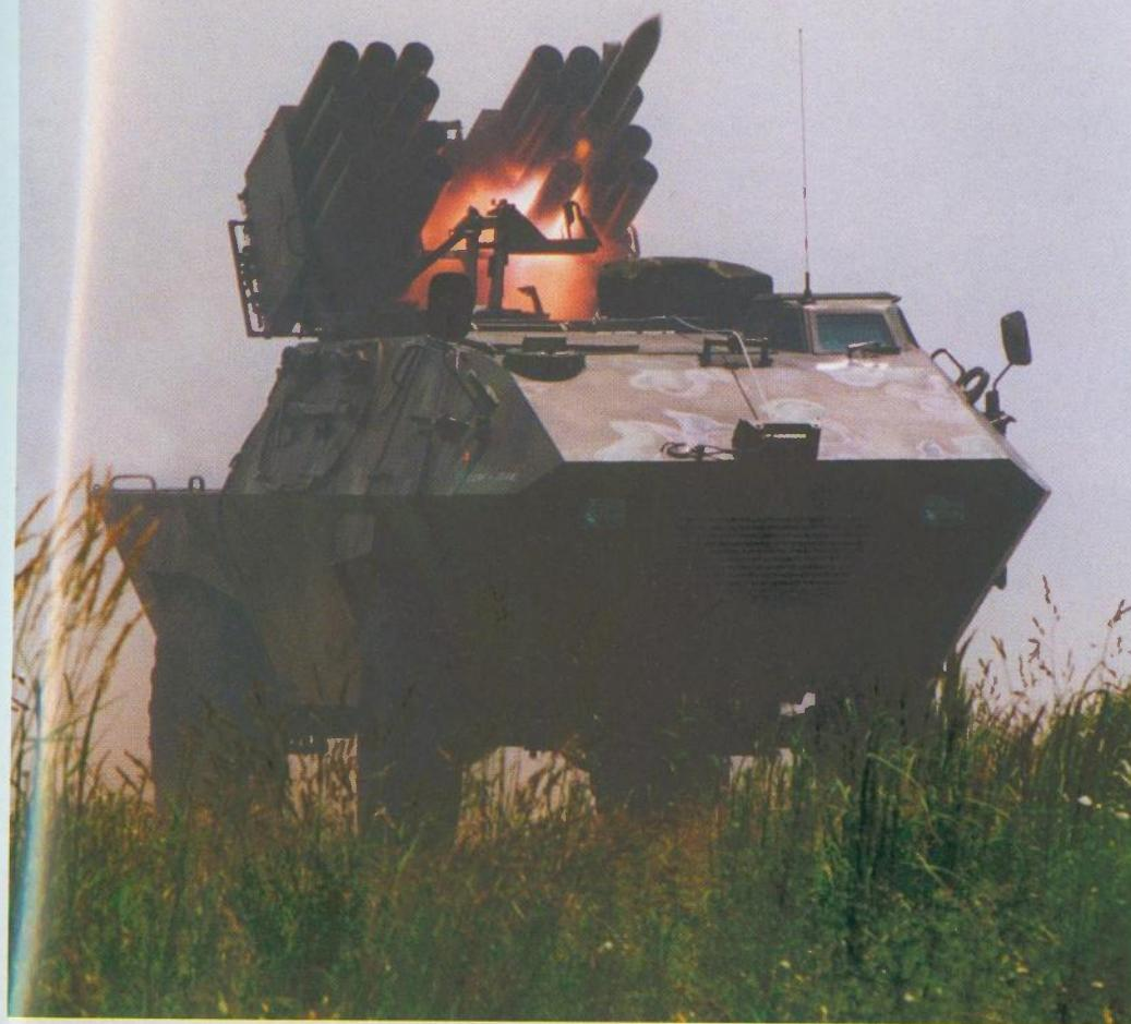
The LOV RAK 24/128 Self-Propelled Rocket Launcher on a light armored wheel vehicle facilitates tactical changes in the firing position.
