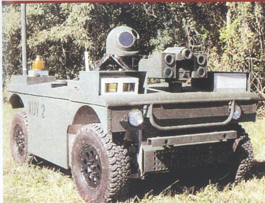
Experimental Unmanned Vehicle (XUV), težak 1150 kg. razvija se u okviru programa Demo III
